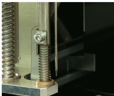
Any adhered substances on the tip of the sample probe are removed.
