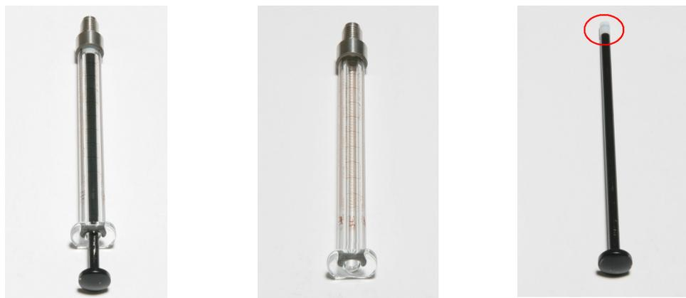
Syringe (Left), Syringe Barrel (Center) and Plunger (Right). The Tip of the PTFE Plunger Seal is Circled
