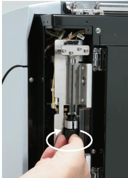
**5** Holding the syringe barrel, turn it in the direction indicated by the arrow, and remove the upper section of the syringe from the instrument.
