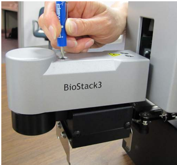
Installing the gripper arm cover
