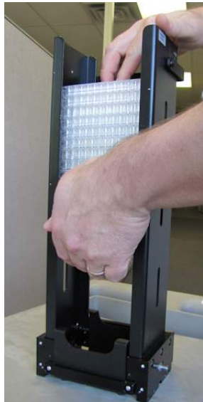
Step 2: Load the plates into the stack on top of pedestal.
