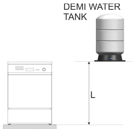
fig. 8 – Tank not under pressure, height with respect to the supporting surface of the device.
