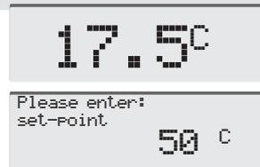
Press the SET key. The setpoint will be shown on the status display. Enter the new setpoint by turning the encoder (e.g. to 50 °C). Confirm your entry by pressing the encoder or the SET key.
