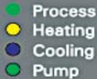
When you press the On/Off key or the power switch to stop the thermoregulation process, all the LEDs will go out.
