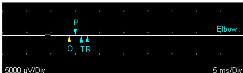
Pattern of auto-cursor placement when amplitude criteria is not met.
