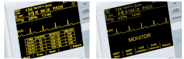
On-screen measurement log and strip-chart recording, document reading and trends.
