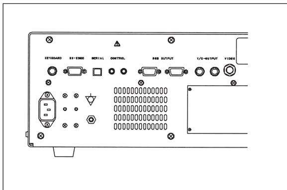
1. Referring to the rear panel diagram, connect a TV monitor and other required equipment such as hard copy equipment, VCR, etc., to the processor.
