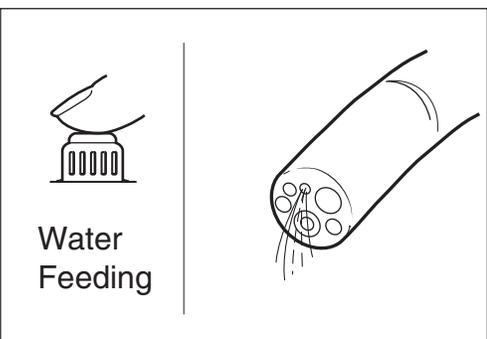
**NOTE** -Use only "fresh" distilled or sterile water for testing of the endoscope air/water delivery functions.
