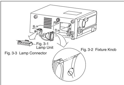
Fig. 3 How to attach a lamp unit
