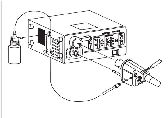
2. Check to ensure that the scope locking lever is open.
