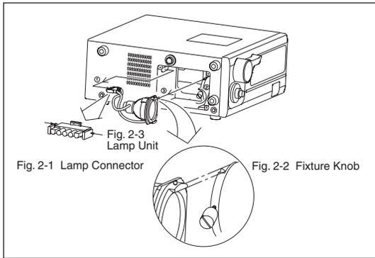
Fig. 2 How to remove the lamp unit
