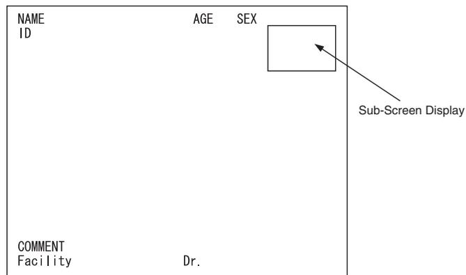
Endoscopic image will be displayed to this area of the monitor screen when freeze function is activated.
