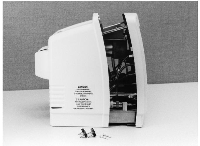
**Removing Chassis from Rear Case**
