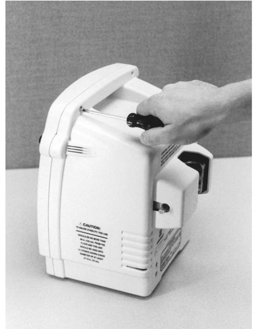
**Removing Chassis from Rear Case**
