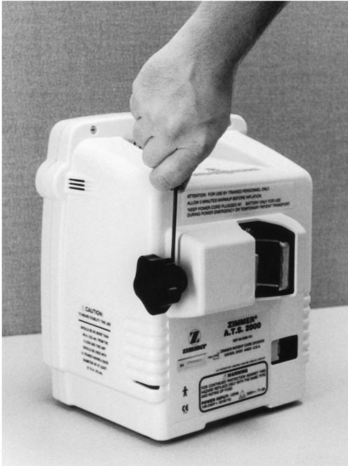
**Removing Chassis from Rear Case**
