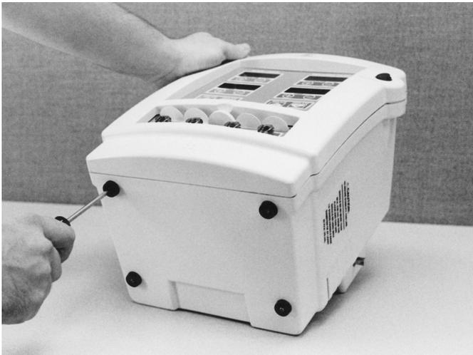
**Removing Chassis from Rear Case**
