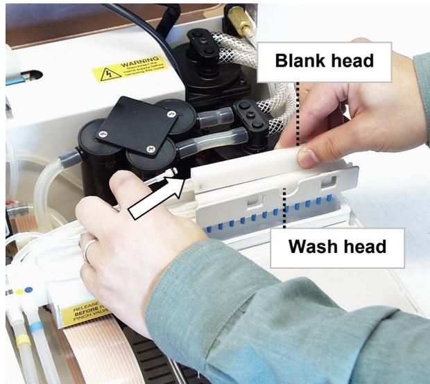
**Fig. 5.26 Fitting the blank head to the rear position**
