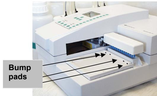
**Fig. 6.2 Plate carrier with four bump pads**
