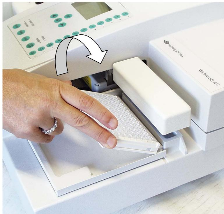
**Fig. 6.3 Inserting the microplate rear first**
