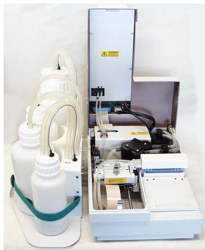
**Fig. 4.2 Wellwash AC front view with the cover open**
