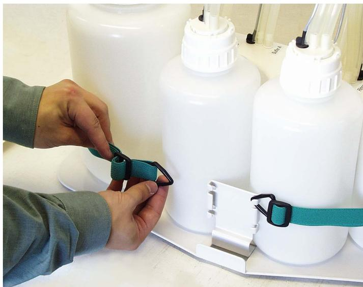
**Fig. 5.17 Adjusting the strap**
