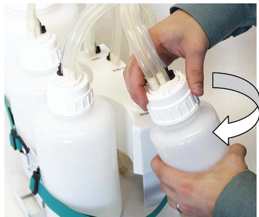
**Fig. 5.13 Tightening the bottle cap**
