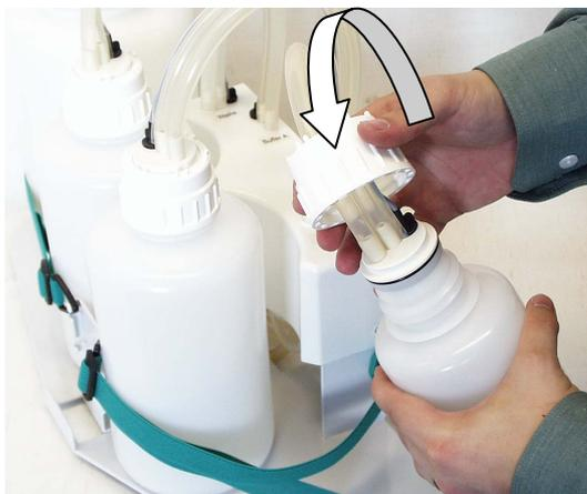
**Fig. 5.12 Reconnecting the bottle cap**
