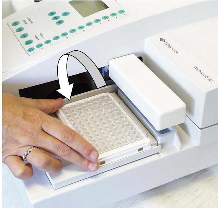
**Fig. 6.4 Lowering the microplate after insertion**
