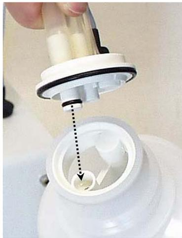
**Fig. 5.11 Mating the plug with the bottle insert**
