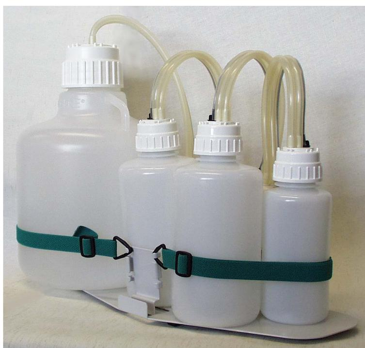
**Fig. 5.21** BMU adjustment piece readjusted for a big bottle
