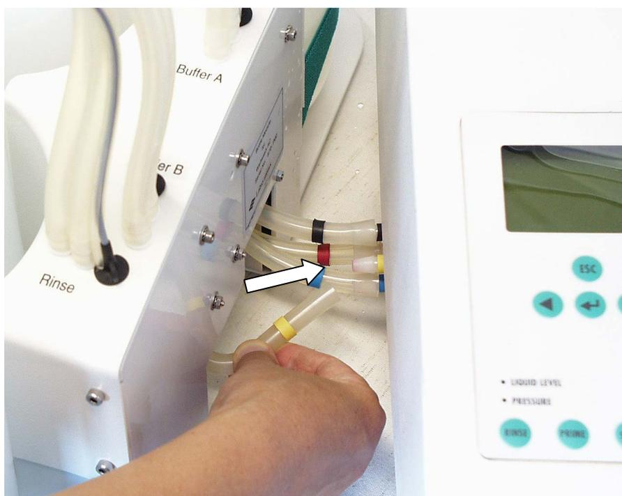
**Fig. 5.9 Connecting the tubing from the BMU to the washer unit**
