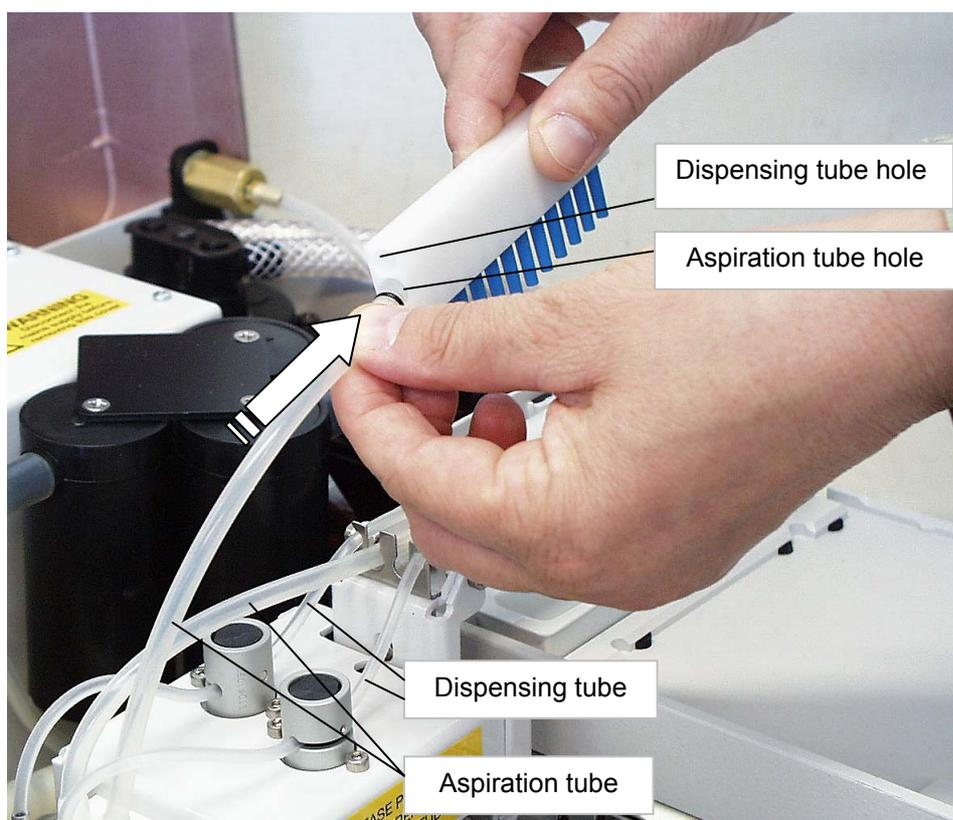
**Fig. 5.22 Fitting the 1 x 12-way wash head to the tubing**
