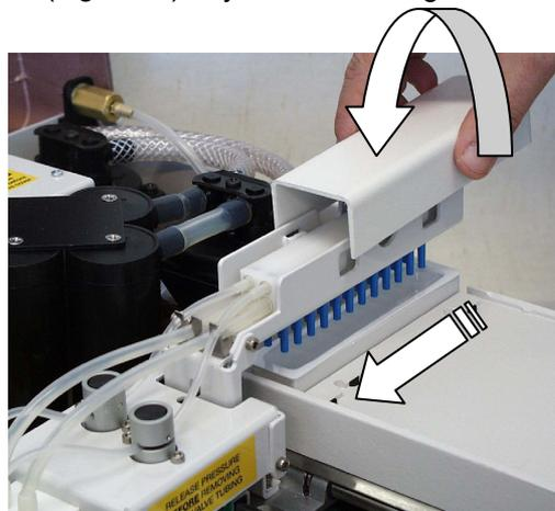
**Fig. 5.25 Fitting the wash head cover back on again**
