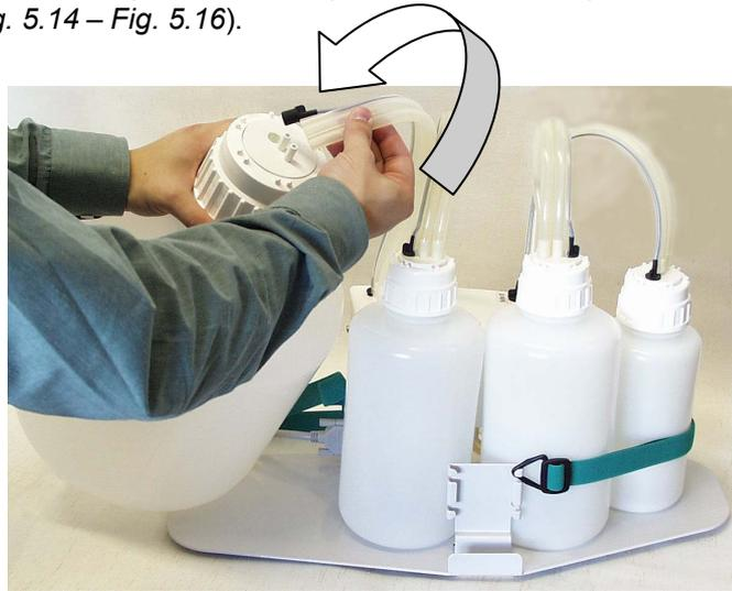
**Fig. 5.14** Connecting the liquid level sensor and the tubing to the cap
