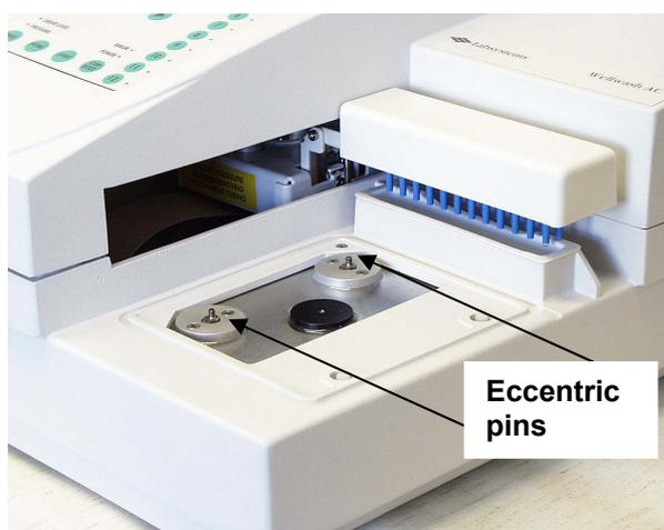
**Fig. 7.2 Eccentric pins of the plate carrier**
