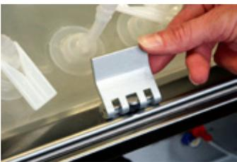
1. Open the guide rails on the bag holder by releasing the lever on both sides of the holder as shown in the figure.
