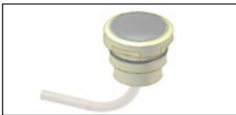
The three-stage, Class A Pt100 resistance thermometer (EN60751) measures the CultiBag RM temperature. The thermometer including the cable is run through the opening into the Bag Holder 20 | 50 and connected to the Rocker 20 | 50 via a plug connection. The head is secured in the opening via an O-ring. Connection to device: Temp 1 and Temp 2, protection class: IP67
