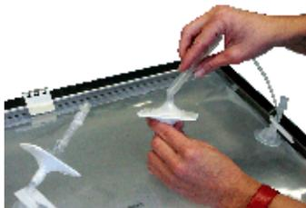
1. Connect the "Gas 1 and/or Gas 2" connection of the BIOSTAT® RM 20 | 50 basic to the sterile exhaust filter on the CultiBag RM using the supplied tubing. (The exhaust filter is the filter without the overpressure valve).
