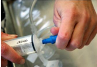
5. Connect the syringe: connect a sterile, single-use syringe without a needle to the Luer connection under aseptic conditions.
