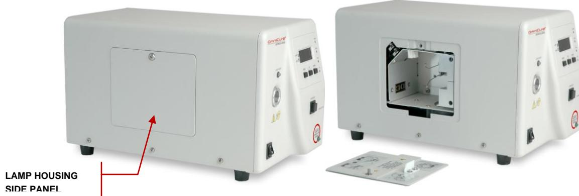
**Figure 3 Lamp Housing Panel**
