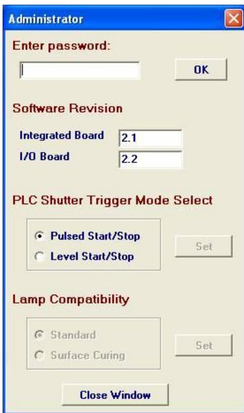
The PLC Shutter Signal Mode can be switched between the pulsed start/stop and the level start/stop without password.
