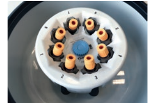
DualSpin rotor with swinging buckets
