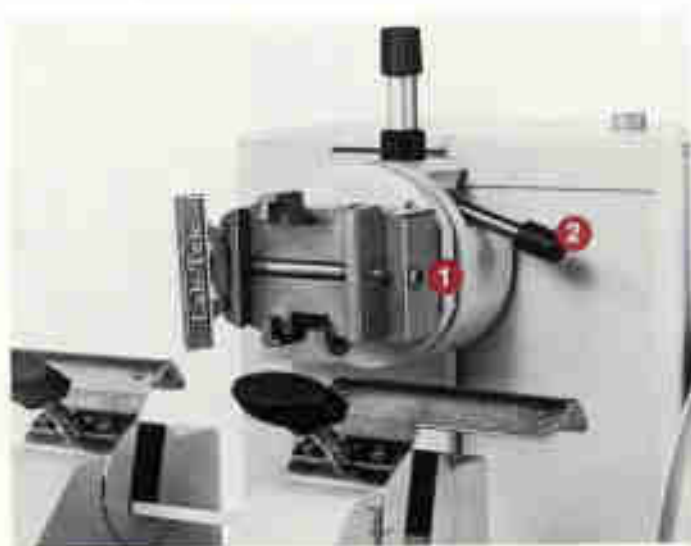
Fig. 11 Lab-Tek adapter in transverse position 1 4mm Allen screw 2 Arresting lever
