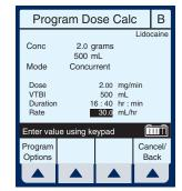
**NOTE:** The Duration field temporarily changes to dashes when the computed value is larger than what can be displayed.
