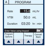
shown in this example, the delivery shows 3 hours and 20 minutes (not 3 minutes and 20 seconds).
