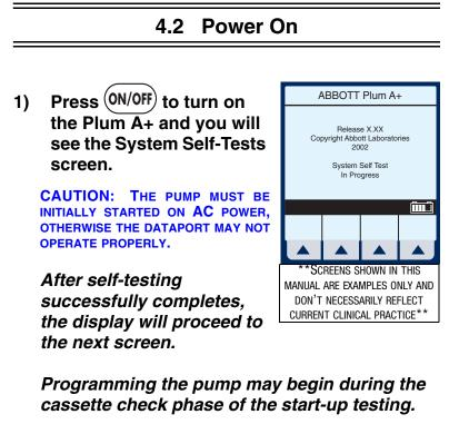
**NOTE:** If battery is missing or defective, a "Battery not installed" message with a "Continue without battery" prompt will appear (AC power only).
