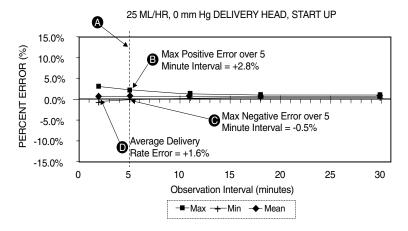
A trained professional can use the resulting graphs to select a pump with the appropriate startup and flow characteristics to suit the clinical application.
