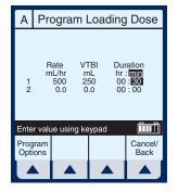
After the values for loading dose Step-1 are entered, use ▼ to highlight the maintenance dose, Step-2.
