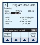
**NOTE:** The Concentration elements and weight value must be entered before the [SELECT] key allows access to remaining fields.
