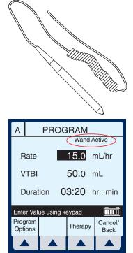
**NOTE:** For Plum A+3, barcode wand is only operational on pump which displays "Wand Active" on screen.
