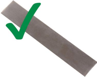
Make sure that the sample is clean and remove any dirt, rust, paint or coating.
