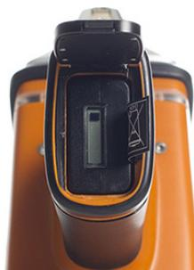
3. Slide the clip at the base of the handle forward to open the battery cover.
