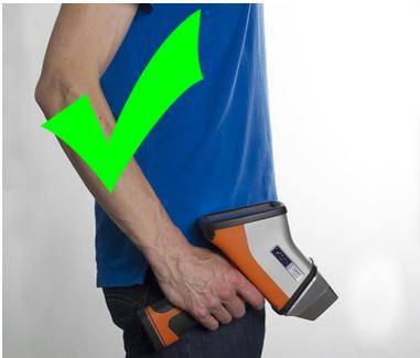
Hold the X-MET8000 series downwards when it is not in use, or put it in the holster.
