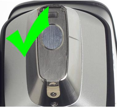
Make sure that the protective film window is intact, and measure sharp objects, in particular metal swarf, with care. It is possible to puncture the protective film window. Refer to: [The Protective Film Window Is Broken](#) on page 116.
