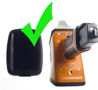
Only remove the battery when the X-MET8000 series is switched off.
