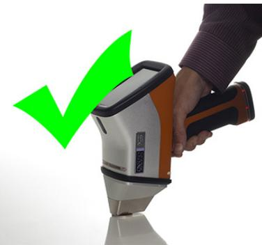
Always place the sample on a flat surface to measure it. Ensure that the sample covers the analyser's measurement window and proximity window.
