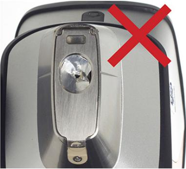
Do not use the X-MET8000 series when the protective film window is broken. Do not press the X-MET8000 series into sharp objects.
