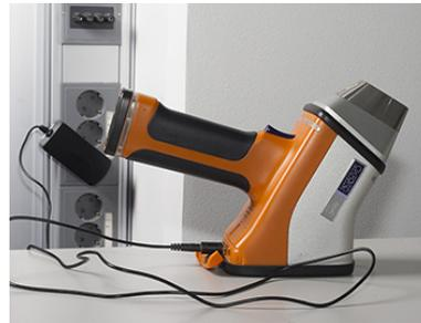
2. Connect the power supply to a mains power supply. Make sure that the mains socket is easily accessible when the power supply is in use.
