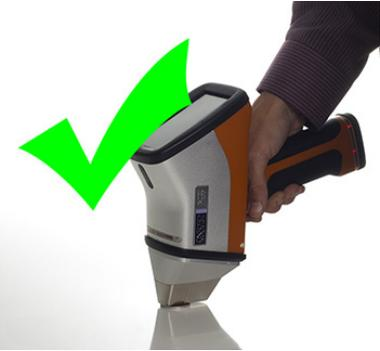
Make sure that the analyser is upright during measurements, and that the nose of the analyser is in full contact with the sample.
