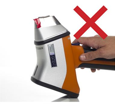
Do not cover the proximity sensor window with a finger, piece of tape, or anything other than the sample.
