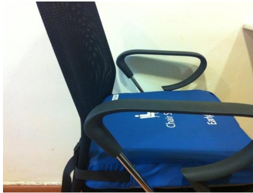
Figure 7: Example of Chair Sensing Unit Strapped to a Chair
