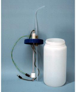
Figure 2.3.1 Assembly of the Electrolyte/Waste System
