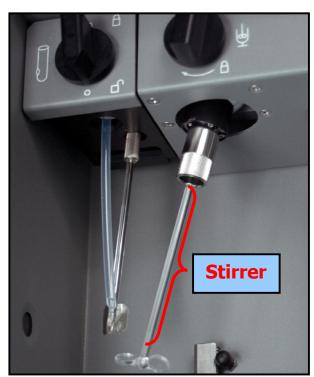
available to the paddles by rotating the collet between finger and thumb. The stirrer must not encounter the electrode or the aperture tube when it rotates.
