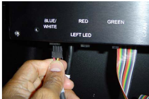
Figure 3.14. Blue/White LED module connector
