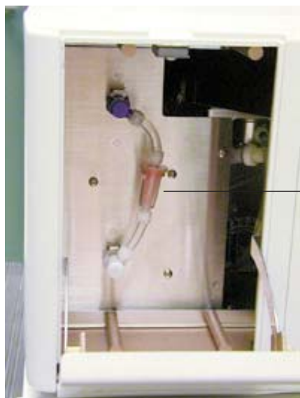
Fig. 3A. Sheath filter internal fluidics features.
