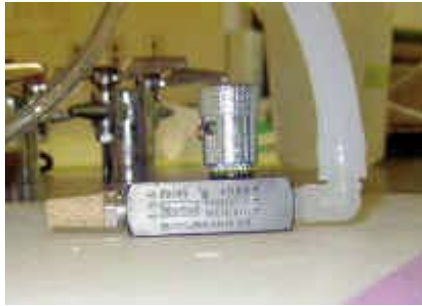
Fig. 23. Gold vacuum control valve.
