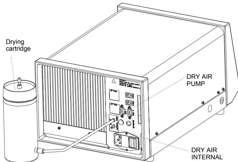
Fig. A - 1 Connections for supplying dry air
