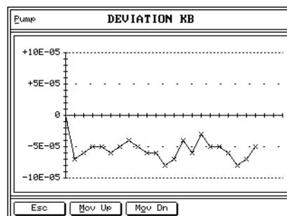
Slight variations of the KB-value are normal. However, after transport a higher offset of the first KB-value with reference to the original KB-value (factory adjustment) is sometimes observed.
