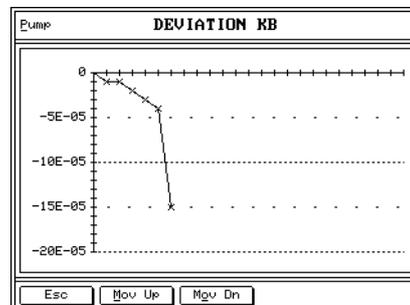
Abrasion of glass from the U-tube oscillator is indicated by the steeply decreasing deviation KB.
