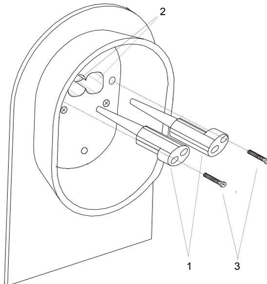
Fig. 5 - 1 Mounting the injection adapters Luer
