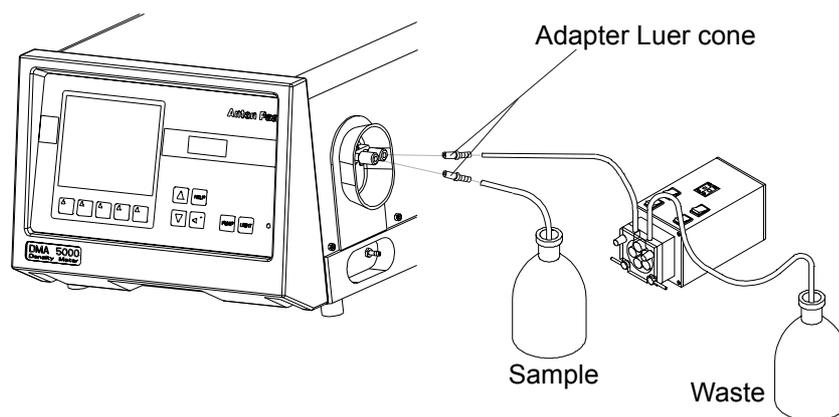
Fig. 9 - 3 Filling, using a peristaltic pump
