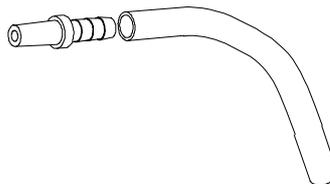
Fig. 5 - 3 Attaching the adapter Luer cone to the hose
