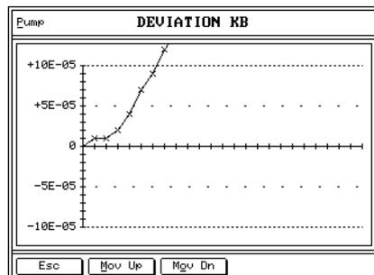
Built-up deposits inside the U-tube oscillator are indicated by the steeply increasing deviation KB.
