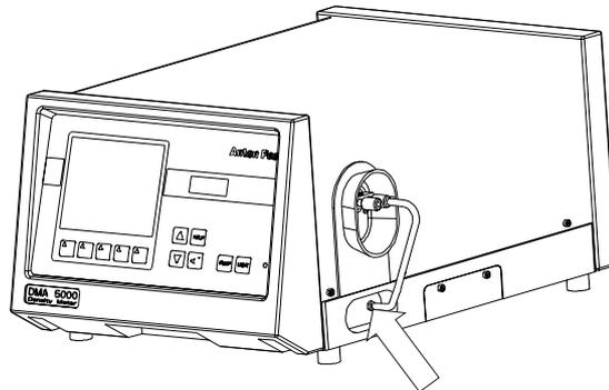
Fig. 5 - 2 Attaching the hose to the air pump
