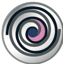
Gas exhausted at center hub
