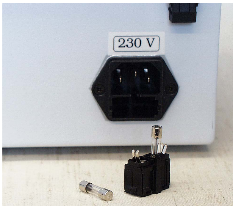
Fig. 7.3 Fuse holder cap with fuses
