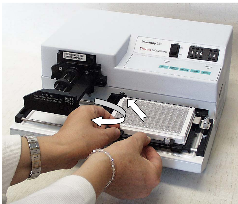
Fig. 6.14 Fastening the front screws of the plate adapter
