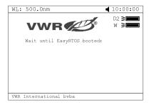
Turn on lamps  $\to$  RAM Check  $\to$  Start RTOS kernel $\to$  Initialize Comm. Port  $\to$  Initialize Printer  $\to$  Initialize AD  $\to$  System position  $\to$  Warm up.
