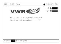
After warm-up, the instrument will ask the user to re-calibrate the system. The user can decide if they need to re-calibrate the system or not. After this step, the instrument is ready to work normally.
