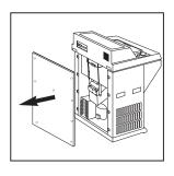
11 Fit the transit plate to the rear of the microtome assembly.
