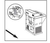
11 Place the spacer between the microtome casting and leadscrew arm (ii). Carefully adjust the leadscrew so that the leadscrew arm rests on the spacer (i). (Note that the leadscrew may need to be manually turned).
