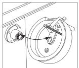
The lever next to the handwheel handle is used to lock the handwheel to prevent inadvertent rotation. To lock the handwheel, push the lever away from you.
