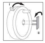
7 Remove the handwheel
