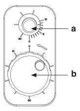
Turn the Rewind/Advance Control knob clockwise to rewind the head and anti-clockwise to advance the head. One rotation of the knob equates to a movement of 100µm at the Specimen Head.
