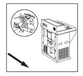
12 Unscrew and remove the nut on top of the defrost valve. Carefully remove the defrost valve from the copper tube and use cable ties to secure it to the transit plate on the rear of the microtome. Place the nut, washer and nameplate into a small bag and secure to the defrost valve.
