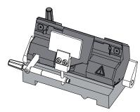
The Knife Holder is constructed of two parts - a Top and a Base. There are three types of Top to suit the types of knife or blade. The same Base supports all versions of Top.
