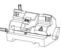
Move the glass plate carefully until the top edge is parallel to the knife. Hold the glass plate firmly in position and tighten up the two screws.
