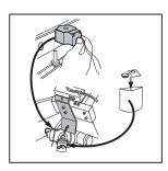
13 Place the wooden supports under the compressor mounting plate.
