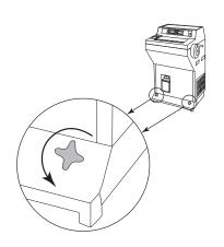
Turn the lowering knobs counter-clockwise until the feet of the instrument are on the floor. The retraction knobs can be unscrewed completely and removed if preferred.
