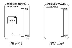
When the instrument is first powered up, the first segment flashes to indicate that the Specimen Head is in its maximum available travel (MAX) position. As the Specimen Head advances at the end of each cutting stroke, the segments of the display light one by one until eventually all the segments are lit when no more travel is available. An audible alarm operates when the end of travel is reached.
