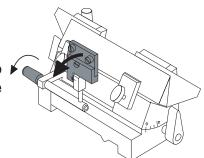
Carefully slide the knife in front of the removable knife guard and place it centrally and squarely in the base of the Knife Holder. Tighten the clamps clockwise to secure the knife in position
