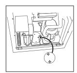
14 Fit and tighten the two red handles to the screws on the base of the compressor mounting plate.
