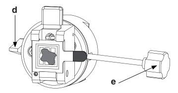
To adjust the up-to-down and left-to-right orientation of the specimen before sectioning takes place, first turn the knob (e) on the end of the adjustment shaft towards you to unlock the movement of the head.
