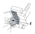
With the coil of the defrost valve still connected to the white wires, place the coil over the tube that projects upward from the copper tube on top of the compressor cooling matrix (g). Unpack the blue plastic components and fit the nameplate, the washer, and then the nut to hold the coil of the defrost valve in position. Fit the plastic plug in the hole in the centre of the rear panel.
