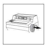
9 Secure the Cryobar with a rubber band. Lift the top cover and secure the window in the closed position using sticky tape. Turn the instrument lowering knobs counter-clockwise to lower the castors to the ground.
