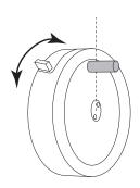
Move the lock lever towards you and check that the handwheel rotates smoothly and produces vertical oscillations of the Specimen Head. Check also that the lock operates at the 'quarter past' and 'half past' the hour clock positions.
