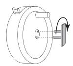
Turn the handwheel until the handle is at the 12 o'clock position then push the lever of the lock away from you. Check that the lock operates and that the handwheel cannot rotate. Check that the Specimen Head is at the top of its travel.
