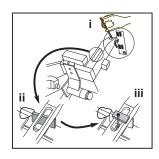
Fit the stud from underneath the leadscrew and secure the top spacer with the 'butterfly' nut.
