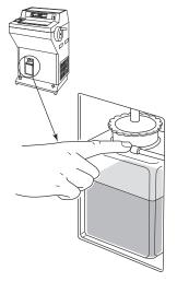
Slide the waste bottle retaining bar to the right, and remove the Waste Bottle. Use a 10% solution of Formalin to fill the Waste Bottle sufficient to cover the outlet tube - approximately 15mm (½ inch) deep. The lid of the waste bottle turns counter clockwise to undo.
