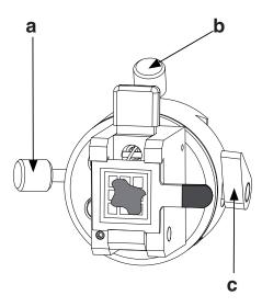
To adjust the up-to-down and left-to-right orientation of the specimen before sectioning takes place, turn the Orientation Clamp towards you to unlock the clamp.
