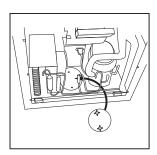
15 Replace the back panel. Make sure the centre bolt is also fitted.
