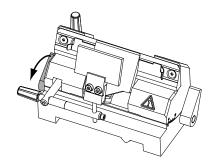
To fit a Knife Holder on the carrier for disposable blades (shown in the diagram), or a standard solid knife, first pull the left hand pivoting lever of the Knife Holder fully toward you.
