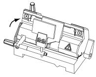
Push the bottom of the Knife Holder away from you, then lock in position by pushing the left hand pivoting lever away from you.
