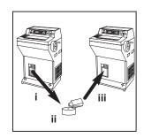
6 Lock the handwheel and remove the handwheel bolt.
