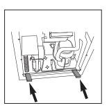
14 Fit and tighten the two red handles to the screws on the base of the compressor mounting plate.
