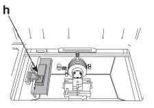
Remove the rubber band and any other packing material from the area around the Cryobar (h) on the left hand wall of the Refrigerated Chamber.
