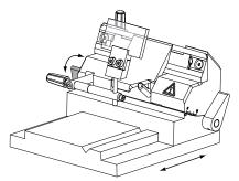
[E only]: Alternatively, if sufficient 'Travel Available' is indicated on the Specimen Travel Indicator, advance the specimen towards the knife using the double chevron (coarse), then the single chevron (fine), push-buttons of the miniature control panel on the left hand side.
