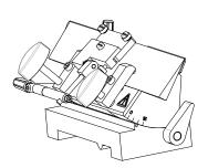
Release the angle clamp by pulling the right hand pivoting lever of the Knife Holder towards you.
