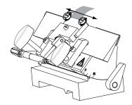
Use the adjusting screw (a) on the anti roll plate support bar to set the approximate height for the anti roll plate. Loosen and tighten the Allen screw as necessary.
