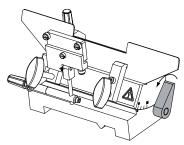
Set the angle of the holder between 4° and 5° (depending on the blade facet angle), then lock it at that angle by pushing the right hand lever away from you.
