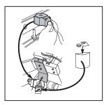
12 Unscrew and remove the nut on top of the defrost valve. Carefully remove the defrost valve from the copper tube and use cable ties to secure it to the transit plate on the rear of the microtome. Place the nut, washer and nameplate into a small bag and secure to the defrost valve.
