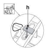
Support the leadscrew arm and use the nylon loop (i) to remove the spacer from between the arm of the leadscrew and the casting of the microtome.
