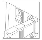
If the protection circuit operates, this will normally indicate a compressor problem. Check that there is adequate space around the outside of the unit for cooling air and that the inlet grill on the right hand side is free of obstructions and dust. Allow 1 hour for the compressor to cool before attempting to reset the trip circuit.
