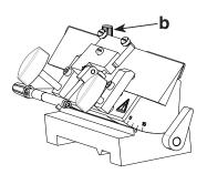
Use the nylon adjuster screw (c) to rectify any slew of the anti roll plate. Make sure that the top of the anti roll plate is parallel with the top edge of the knife/blade.
