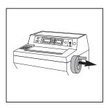
8 Secure the Cryobar with a rubber band. Lift the top cover and secure the window in the closed position using sticky tape. Turn the instrument lowering knobs counter-clockwise to lower the castors to the ground.
