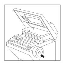
Raise the front edge of the top cover, remove the transit packing from the top of the sliding window, then lower the cover back into position. Push open the sliding window to gain access to the Refrigerated Chamber.
