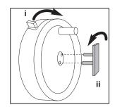
7 Remove the handwheel
