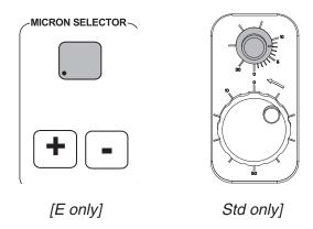
To cut sections, turn the Handwheel smoothly. The instrument performs a single cutting stroke with each full revolution of the Handwheel and cuts a section of the specimen.
