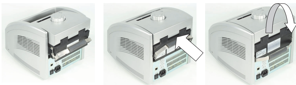
Figure 4–9. Installing a block in the Arktik base unit
