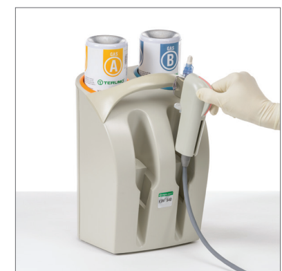
The cable head, with sensor attached, is placed in the calibrator.
