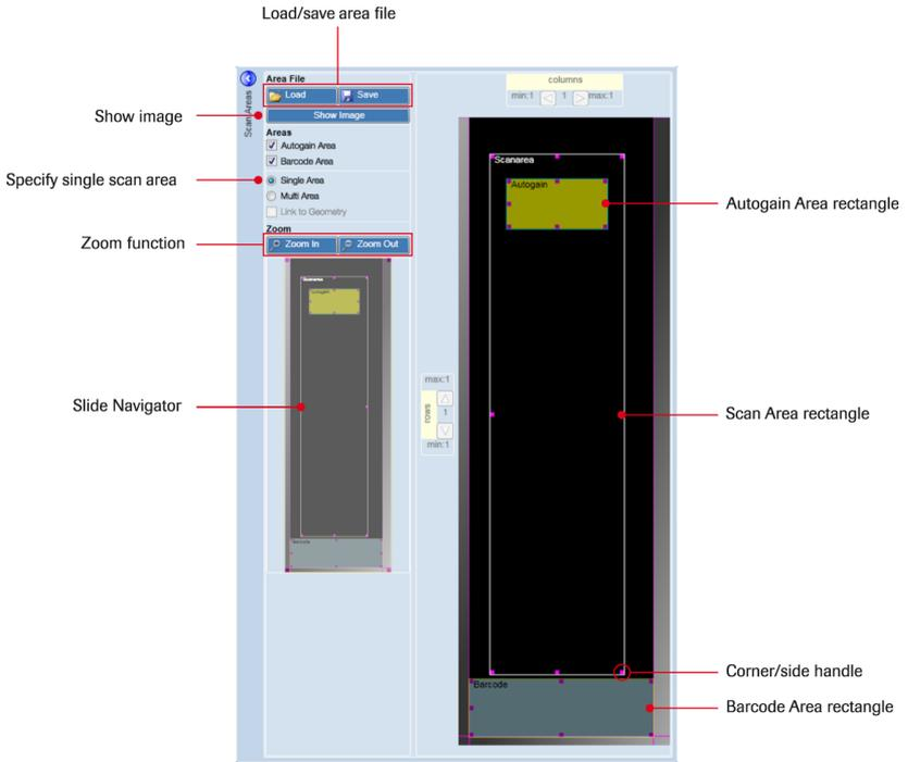
**Figure 28: Area Definition Control for Specifying a Single Scan Area**
