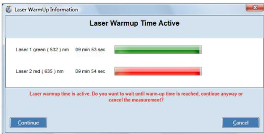
**Figure 31: Laser Warmup Time Active Window**
