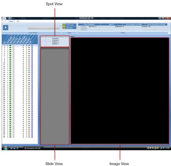
**Figure 19: Components of the Instrument Software Workspace**
