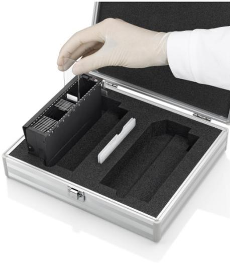
**Figure 9: Inserting Slides into the Slide Magazine (Horizontally in Box)**
