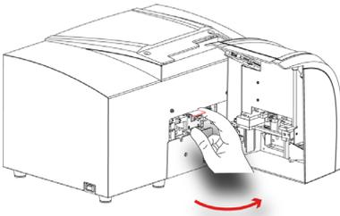
**Figure 41: Removing the Slide from the Slide Transport**
