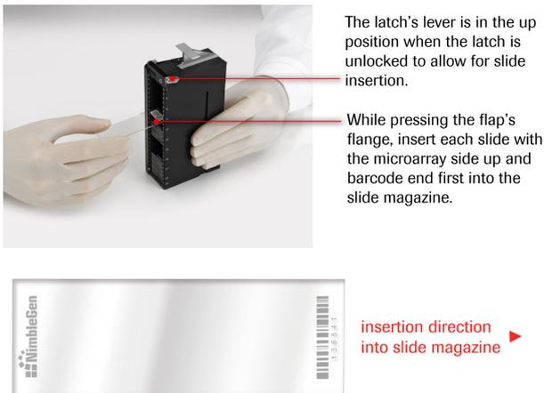
**Figure 8: Inserting Slides into the Slide Magazine (Upright)**
