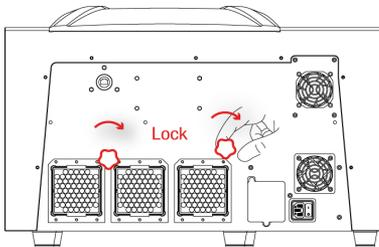
**Figure 43: Tightening the Stacker Locks**
