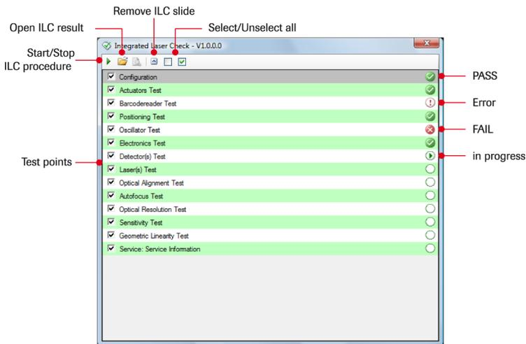
**Figure 16: Integrated Laser Check Window**
