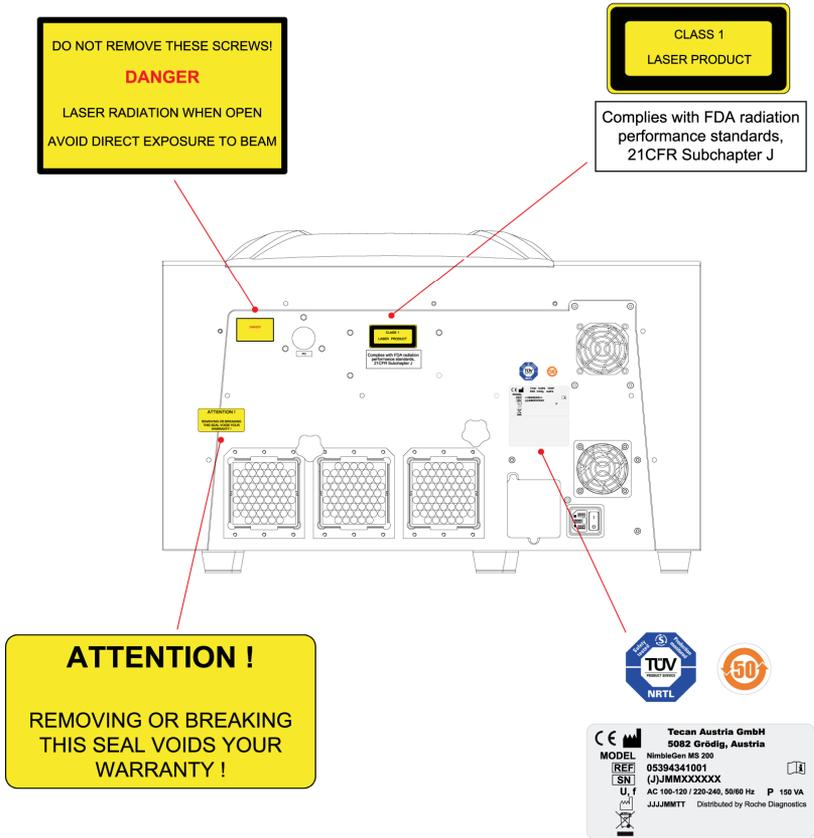
**Figure 1: Safety and Warning Labels on the Microarray Scanner**
