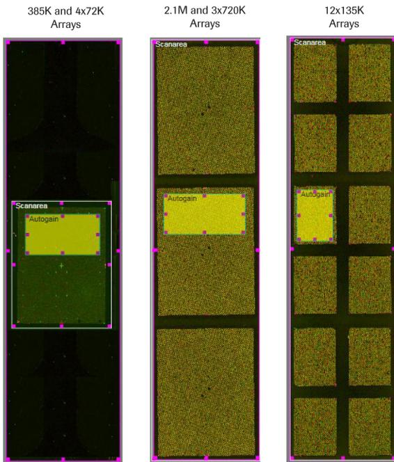
**Figure 30: Examples of Setting the Autogain Area for NimbleGen Arrays**
