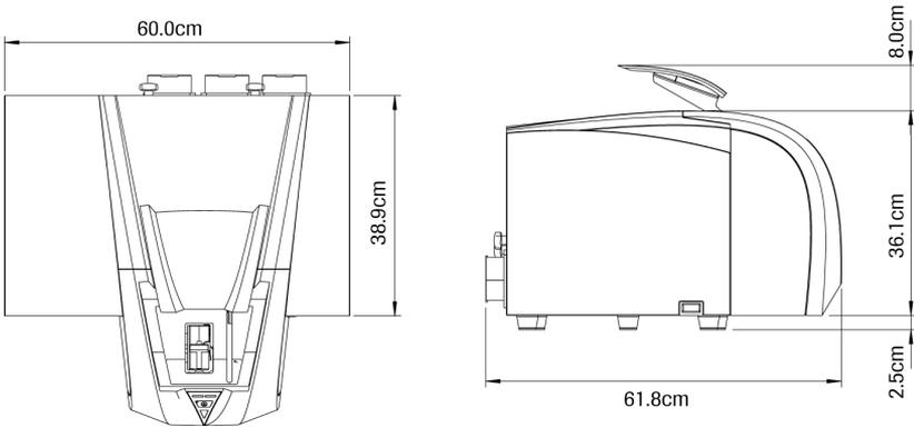
**Figure 12: Dimensions of the Microarray Scanner (Top View and Side View)**
