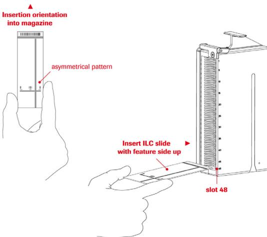
**Figure 17: Inserting the ILC Slide**
