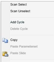
3. Highlight the rows for the slides to process using the same parameters, right-click, and select **Paste Parameter Settings** from the menu.
