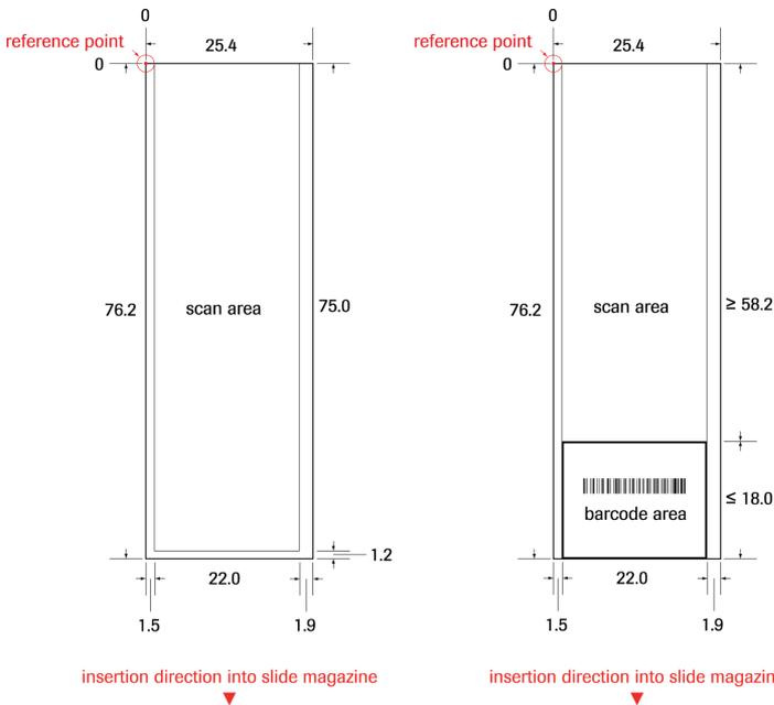
**Figure 2: Scan Area Dimensions (in mm) on Standard Slides with Maximal Barcode Area Definition**
