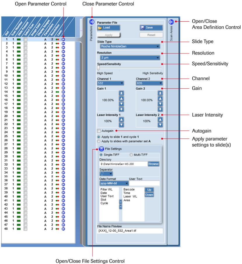
**Figure 25: Magazine Control (Left) and Parameter Control (Right)**
