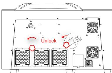
**Figure 39: Unlocking the Stacker Locks**
