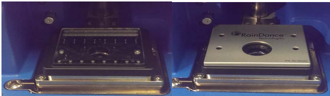
Figure 5-9: Placing the Chip Compression Plate
