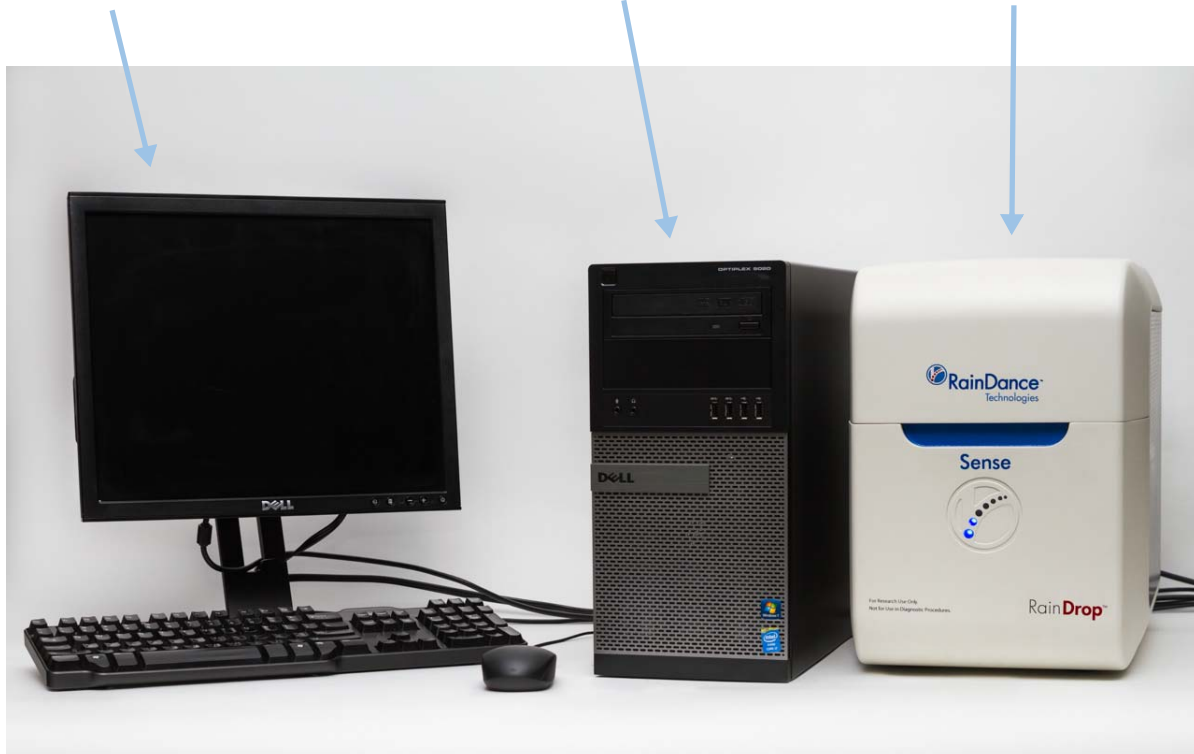
Figure 2-2: RainDrop Sense Major Components
