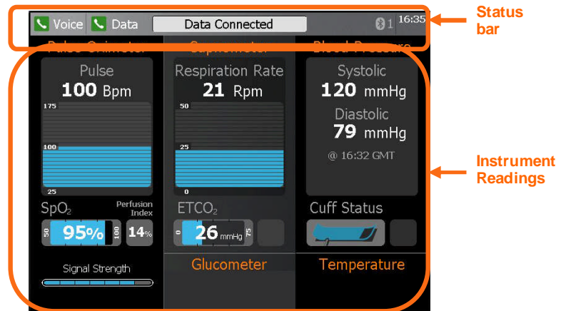
Example of the Tempus IC Screen Display
