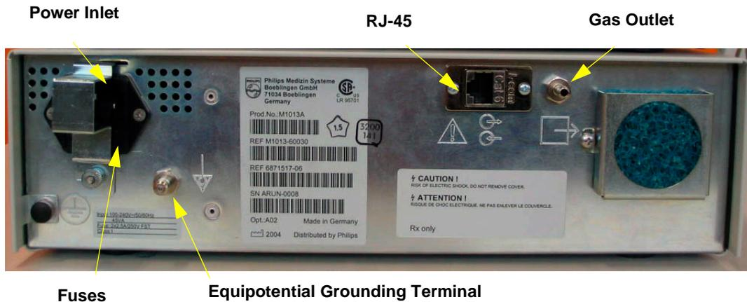
The RJ-45 connector is the interface connector for the Philips IntelliVue patient monitors.
