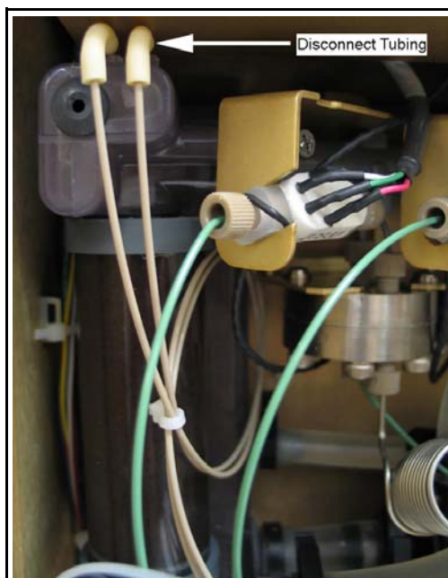
Figure 46: Disconnect the Tan Tubing that Connects to the DI Water Reservoir
