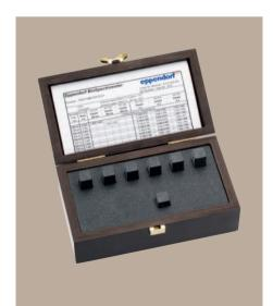
The secondary UV/Vis reference filter set is used to verify the photometric and wavelength systematic errors according to NIST (National Institute of Standards and Technology, Gaithersburg MD, USA).
