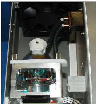
**Figure 21. Lift Bulb Mounting Bracket**
