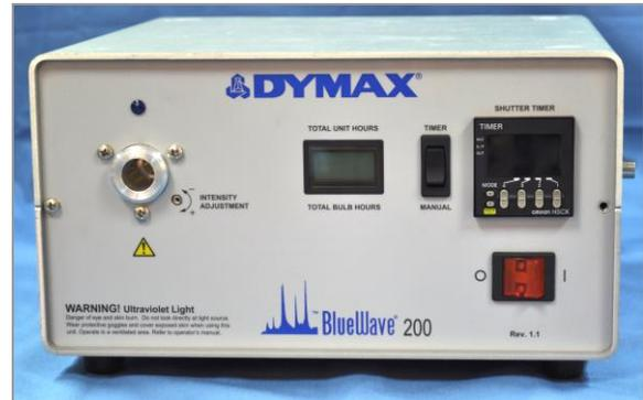
**WARNING!** Always engage the lightguide in the lightguide mount before the system is turned on. Also remove the lightguide from the lightguide mount **ONLY AFTER** the light is turned off to avoid the possibility of exposure to the light. Lightly tighten the setscrew for safety.
