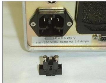
**Figure 19. Fuses Removed from Holder**
