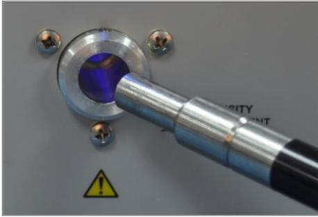
6. If desired, the Lightguide may be fastened into place by lightly tightening the securing Setscrew installed in the Lightguide Mount. A hex wrench is provided with the *BlueWave 200* for this purpose. The Setscrew should be tightened gently to prevent damaging the Lightguide.
