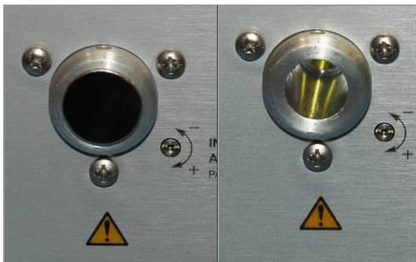
4. Remove the protective end caps from the Lightguide. Visually inspect the two ends of the Lightguide to verify that no foreign material is present. The ends of a Dymax liquid-filled Lightguide can be cleaned with isopropyl alcohol as required to remove foreign material and deposition from outgassing.
