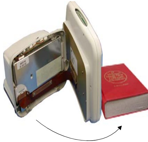
Display assembly with metallic display shield
