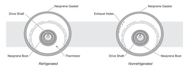
Figure 1-2. Interior View of the Centrifuge
