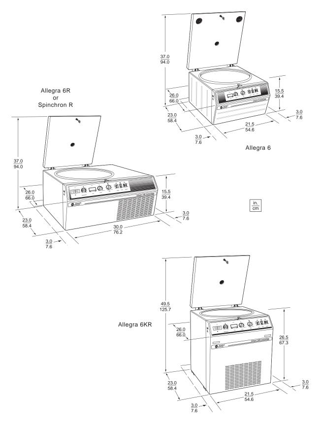
Figure 2-1. Centrifuge Dimensions
