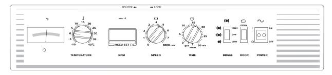
Figure 1-4. The Control Panel (Refrigerated Models)
