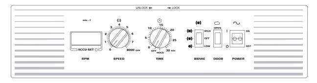
Figure 1-3. The Control Panel (Nonrefrigerated Model)
