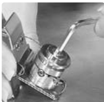
Step 3: Remove the cell screw and remove the gasket
