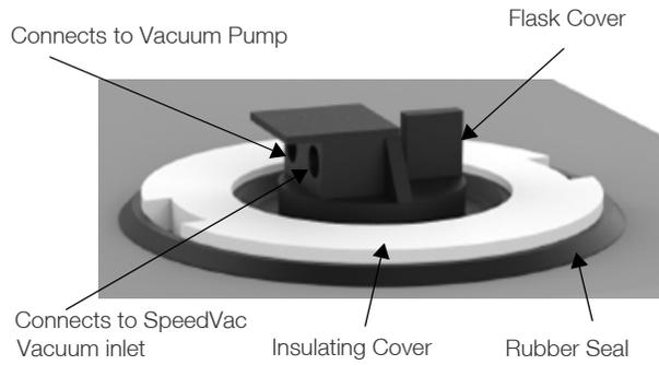
5. Align the circular groove of the Flask Cover with the mouth of the Glass Condensation Flask. Press firmly into place to make a good seal.
