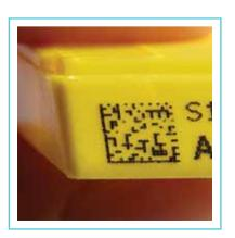
Print 2D Data Matrix barcodes on cassettes to automate sample identification in downstream processes.
