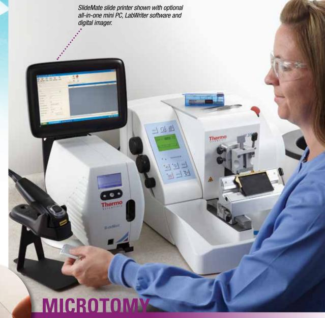
Slides are printed on-demand during sectioning at the microtome.
