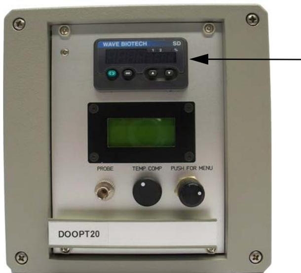
**Figure 3-1.** Example of stand-alone instrument (DOOPT20) with a small Process controller, see arrow.
