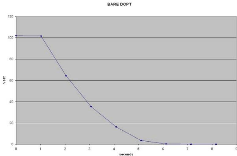
The graph below shows the response time going from 0% oxygen to air saturation. The response time ( $t_{90}$ ) is about the same (4 to 5 seconds).
