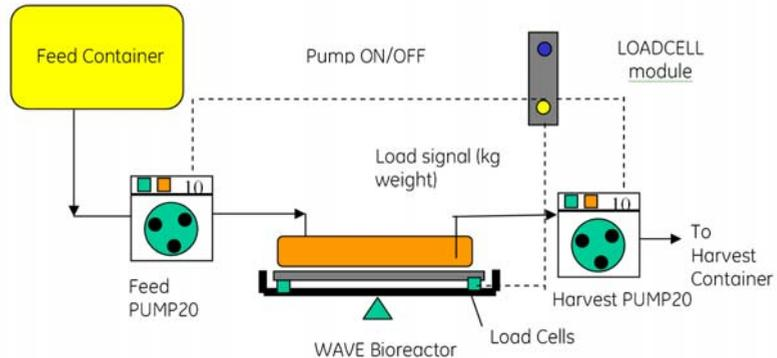
When used with a LOADCELL equipped WAVE Bioreactor 20/50, PUMP20 can be automatically switched on and off to deliver a set feed rate or controlled harvest. When used with a shorting plug, PUMP20 can be used as a variable speed standalone pump.
