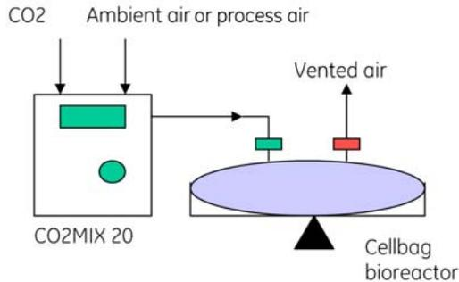
**Figure 5-1.** Diagram of CO2MIX20 connected to the base unit.
