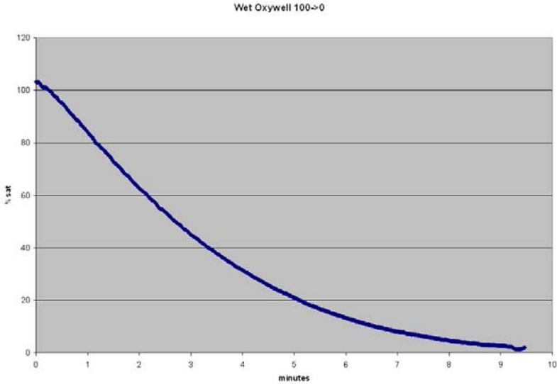
In a dry Oxywell2 the response time is quite long due to the relatively large amount of stagnant air in the tip that must diffuse through the silicone. The response time ( $t_{90}$ ) can range from 5 to 6 minutes as shown in the graph below.
