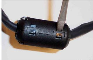
3. Place the ferrite around the new power supply cable 2 inches (+/- 1/2 inch), from the 5 pin din connector.
