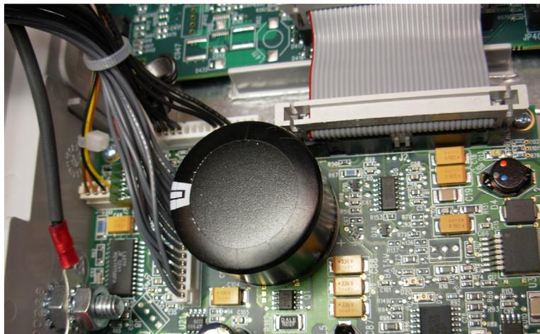
3. Disconnect the cable connectors on the power supply board.
