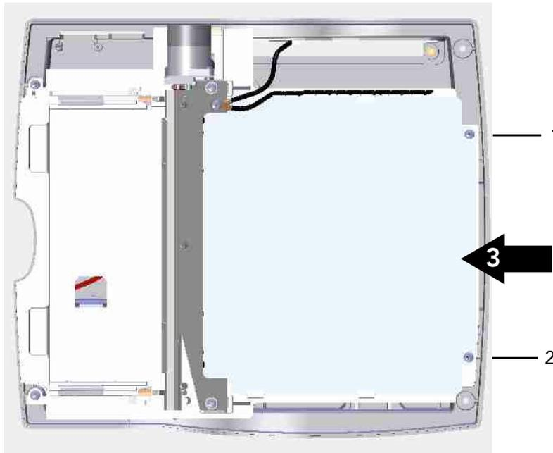
2. Lift out the paper drive assembly and rotate clockwise 180° to set aside.
