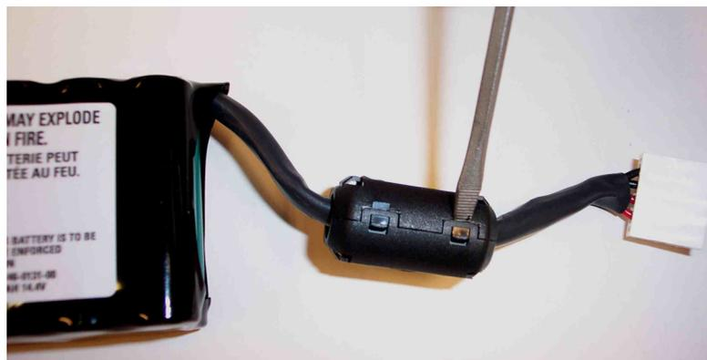
**Figure 4-1: Example of ferrite removal for the Burdick 8300**
