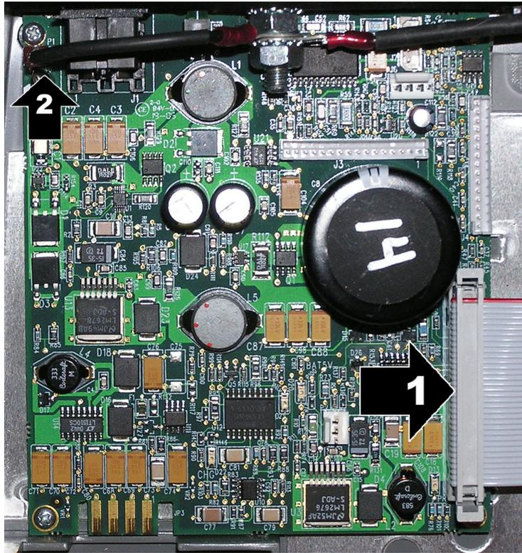
**Figure 4-3:** Power supply board removal
