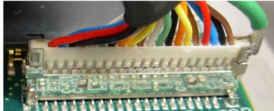
**Figure 4-2: Video cable installation**
