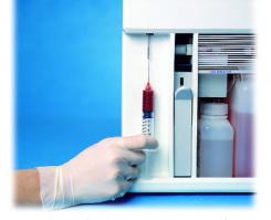
Easy sampling: Present a sample to the sipper tube and press the keypad. The 2300 automatically aspirates the sample and, in less than 60 seconds, displays and prints glucose and lactate levels.
