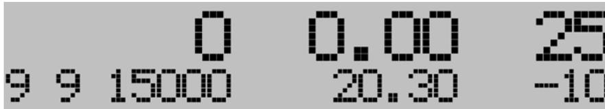
The top line shows the speed and the time. Both lines display **0**. The temperature indicator displays the current temperature inside the rotor chamber. The bottom line shows the values for the last run.
