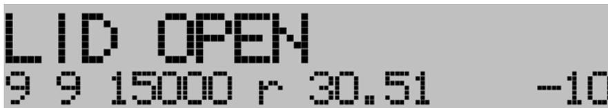
The top line shows the message **lid open**. The bottom line shows the values for the last run.
