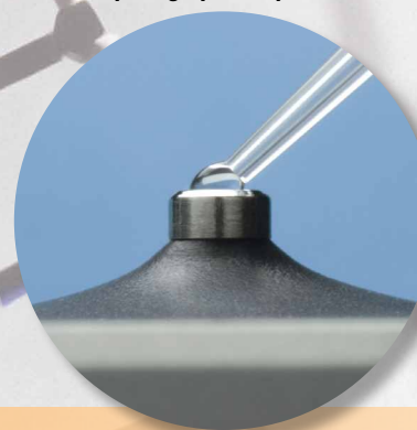
Pipetting 1 \mu L onto pedestal
