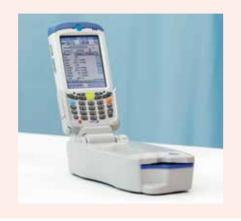
Handheld wireless solution that provides blood gas, electrolyte, and metabolite results at the patient's side.
