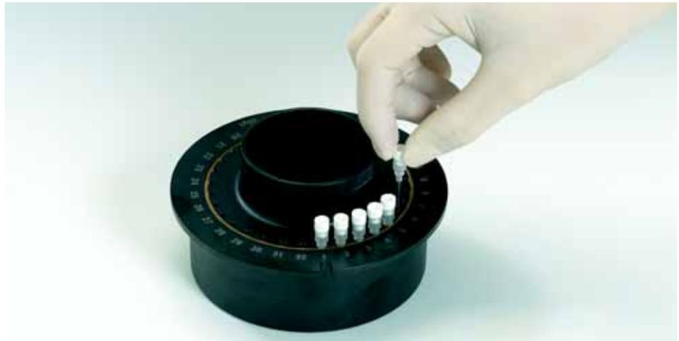
**!** When pressing the capillaries into the LightCycler® 2.0 Sample Carousel, do not press too hard. Do not use LightCycler® capillaries that show slight cracks or cracked slightly during insertion into the LightCycler® 2.0 Sample Carousel. Do not use LightCycler® capillaries that fell down. LightCycler® capillaries with slight cracks, possibly invisible, might crack during a LightCycler® run.
