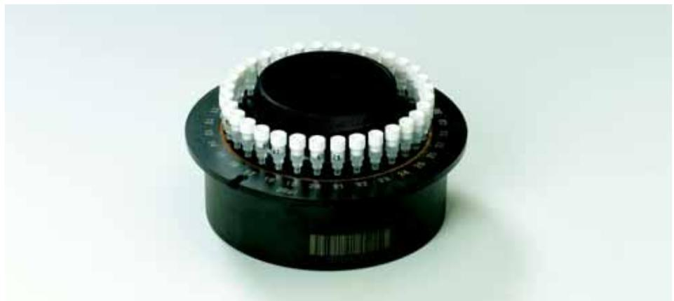
Once the loaded carousel is placed on the LightCycler® Capillary Releaser and pushed down using the flat of your hand, the capillaries are released from being firmly held by the rubber O-ring, and held at a slightly elevated position, allowing easy removal of the capillaries from the sample carousel.
