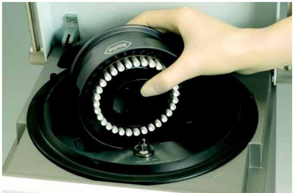
**?** Alternatively, you can spin down the reaction mix within the capillaries with the help of the LightCycler® Centrifuge Adapters in a standard benchtop centrifuge, like the Biofuge 19 from Heraeus Instruments, briefly at not more than 735 x g. Take care to use only rotors that are designed to hold 2.0 ml reaction tubes.
