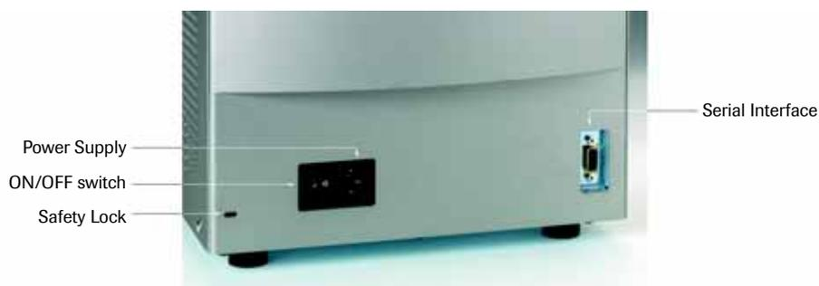
Rear connections of the LightCycler<sup>®</sup> 2.0 Instrument
