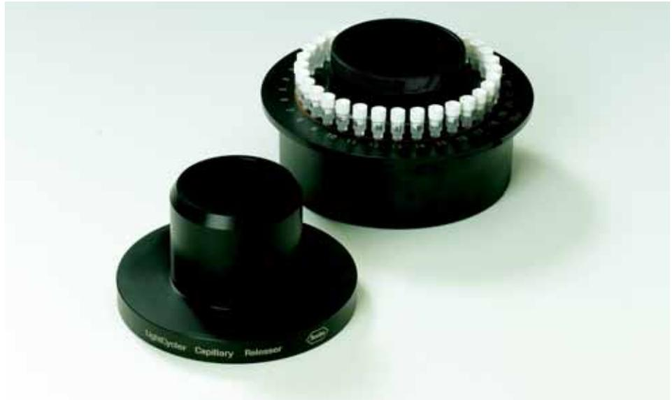
The LightCycler® Capillary Releaser is a plastic part, slightly smaller in diameter, than the sample carousel. It is used for the easy unloading of capillaries from the LightCycler® 2.0 Sample Carousel.
