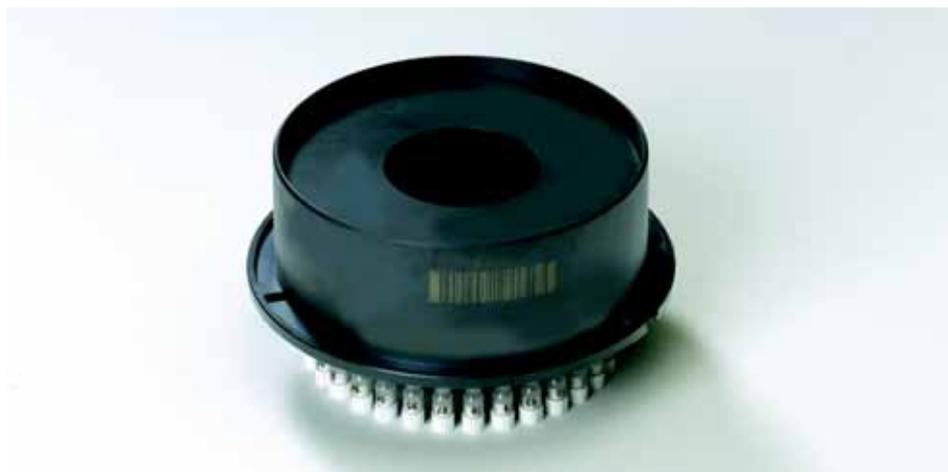
When the capillaries are simply to be discarded, the loaded sample carousel may be put onto the table upside down. The LightCycler® Capillary Releaser is then inserted and pressed down to release the capillaries.
