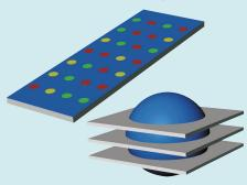
The non-confocal optical path in GenePix 4100A Scanners is designed specifically for microarrays. Confocal optics do not benefit microarray imaging, because the primary source of background is in the same plane of focus as the sample (left). Confocal imaging is primarily beneficial for rejecting out-of-plane background when scanning a thick sample (right).
