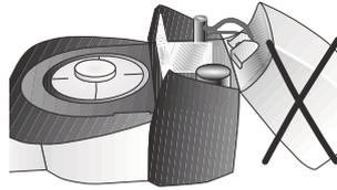
The furnace head should not be removed from the furnace base as long as the furnace head is connected by means of the heater cable.
