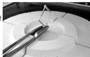
4. If necessary, use the furnace tongs to apply slight pressure to the center of the calibration base until the calibration sample clicks into place. Observe the corresponding markings.
