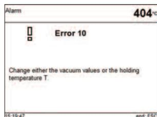
The error group symbol should supply a first indication of the type of error (entry error = exclamation mark; technical error = fork wrench; Note = "i" symbol) without the user having to consult the Operating Instructions.
