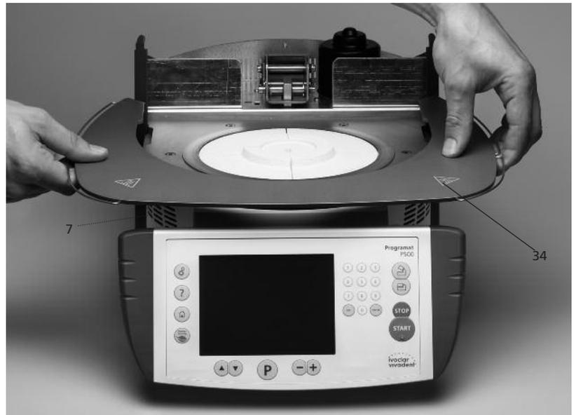
Secure the cooling tray (34) with the two screws (35) including the silicone washer (47).
