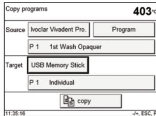
All the existing firing programs (Ivoclar Vivadent or individual programs) of the furnace can be saved on a prepared memory stick. Select Selection – Program Manager – Copy programs and make a choice using the +/- keys:
