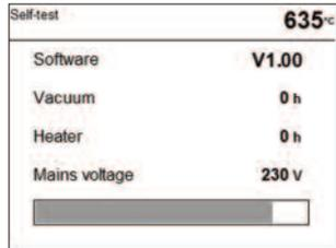
Put ON/OFF switch (11) on position "I". The furnace conducts an automatic self-test, which will be indicated in the beginning. Subsequently, a status bar shows how many % of the self-test have been completed. Make sure that the furnace is not manipulated during this time.
