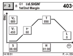
Each program can be directly selected by its program number. The program number is shown in the upper left area of the program display (e.g. P95). To quickly select a program, press the P key and enter the program number. Confirm with the Enter key.
