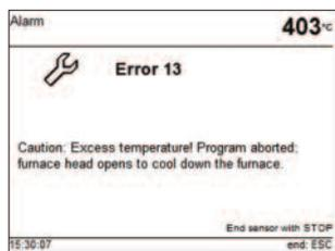
The furnace continuously checks all functions during operation. If an error is detected, the respective error message is displayed.
