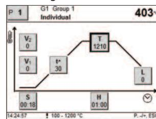
If an illogical value is entered by means of the numeric keys (outside the current value range), the invalid entry still blinks after confirmation.
