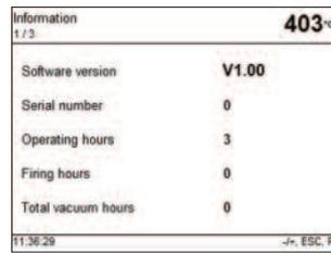
The information pages 1 to 3 provide information on the current software version, operating hours, calibration settings and status of the identified USB devices, such as printer and USB memory stick. The information display also serves to check whether the Programat furnace has identified a USB device.
