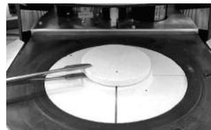
3. Carefully grip the upper part of the ATK 2 using the furnace tongs (Caution: Fracture risk of the ceramic) and insert it into the holes designated for this purpose until it snaps into place.
