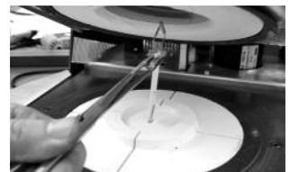
7. Replace the firing plate using the furnace tongs.
