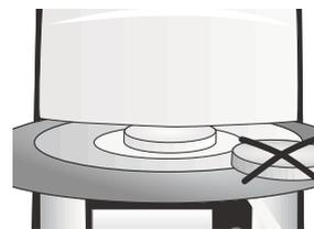
Firing trays must not be placed in the area surrounding the firing table, since this will obstruct the closing of the furnace head.
