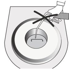
This product contains ceramic fibres and may release fibre dust. Do not use compressed air, or blow, on the furnace thus distributing the dust in the environment and observe the additional notes on page 11.
