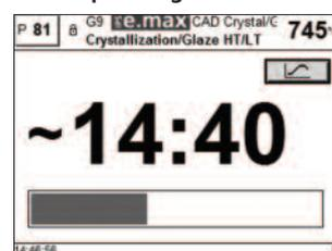
Pressing the "Time" touch button in the firing curve display switches the view to the remaining time indicator.
