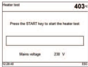
The quality of the heating muffle may be automatically checked by means of the heater test (duration: approximately 7 minutes). The heater test should only be conducted with the empty firing chamber, since an object in the chamber (e.g. firing tray) may influence the test result. Conduct the heater test immediately after
