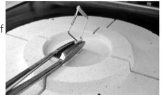
4. If necessary, use the furnace tongs to apply slight pressure to the center of the calibration base until the calibration sample clicks into place. Observe the corresponding markings.
