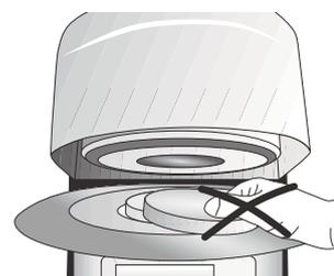
Never place objects in the firing chamber by hand, since there is a burn hazard. Always use the tongs (accessories) supplied for this purpose. Never touch the hot surface of the furnace head, as there is a burn hazard. Please also refer to the warnings on the furnace.
