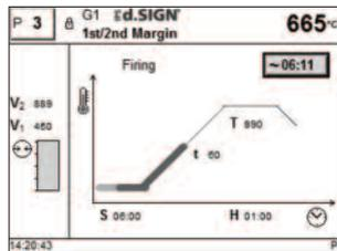
Press the START key (73) to start the program. The green Start LED starts flashing. The process is indicated in the firing curve display.
