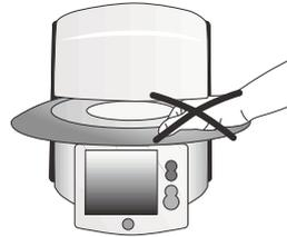
Never reach under the furnace head with the hand or other parts of the body during operation, since there is a risk of crushing and a burn hazard.
