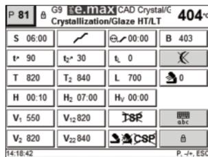
If the cursor is positioned on the "one-stage symbol" and the symbol is switched to the "two-stage symbol" by pressing the + or - key, the program has been set to "two-stage".
