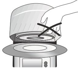
The furnace has an electric drive and must be operated by means of the electronic controls. Never open the furnace head by hand, since the mechanism will be damaged.
