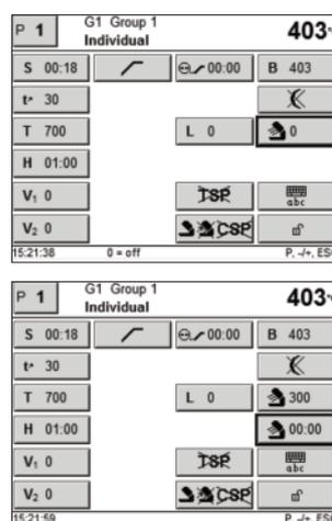
For a program with individually activated pre-drying, the desired "pre-drying temperature" is set after the program start with the furnace head open (heating or cooling). Once this temperature is reached, pre-drying is carried out during the "pre-drying holding time". Once the holding time has elapsed, the furnace head is closed within the desired closing time.
