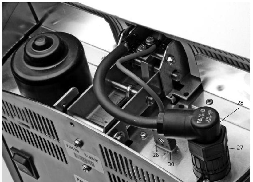
Secure the heater plug (28) with the plug fuse (27) by turning it until the heater plug (28) has been secured.
