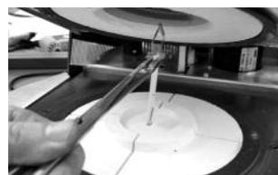
7. Replace the firing plate using the furnace tongs.
