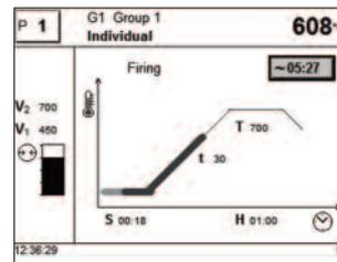
Press the START key (73) to start the program. The process is indicated in the firing curve display.
