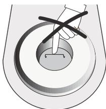
Do not touch the thermocouple or the quartz tube in the firing chamber. Avoid contact with the skin (grease contamination), as the parts may be damaged.
