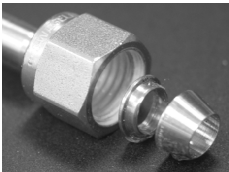
Figure E-2: Correct Orientation of Nuts and Ferrules
