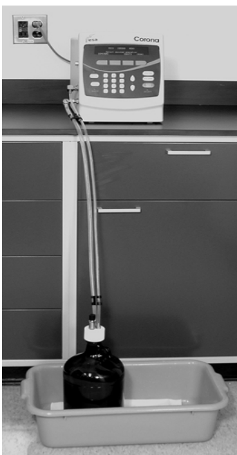
Figure 2-9: Correct Setup of Drain Tubing
