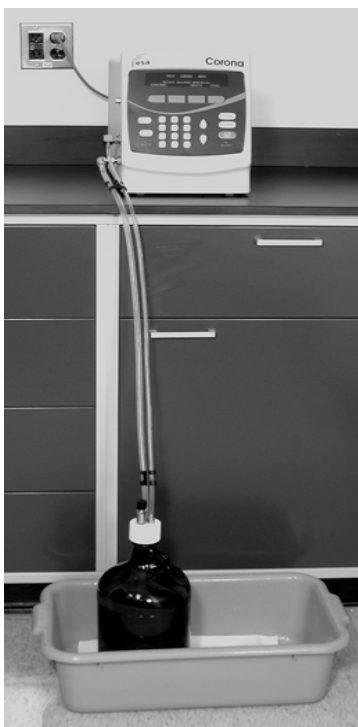
Figure E-5: Correct Setup of Drain Tubing
