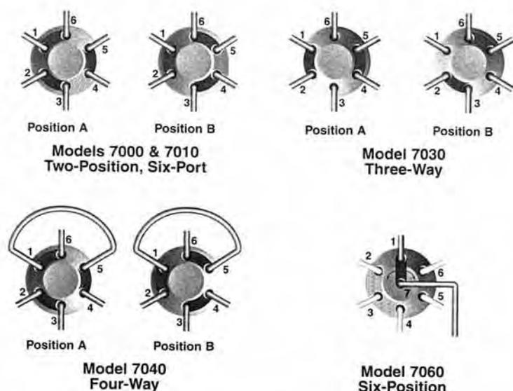
Fig. 1. Flow diagrams of Rheodyne Type 70 high pressure switching valves.
