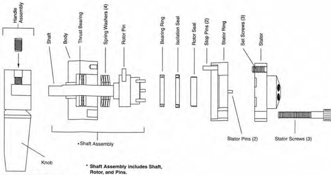
Fig. 4. Exploded view of Type 70 valves.
