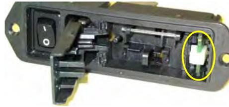
Fig. 5: Voltage selector board
