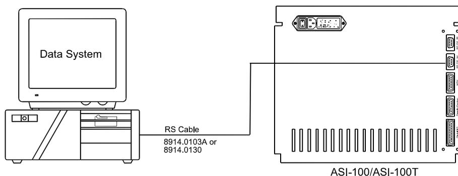
Fig. 10: Direct connection via RS-232
