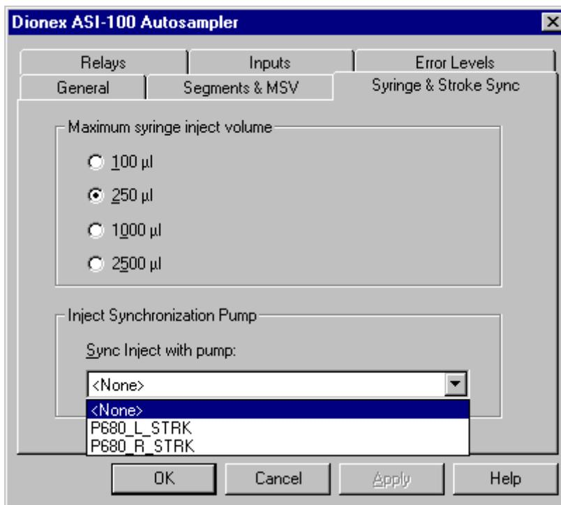
Fig. 25: Syringe & Stroke Sync tab page (In this case, a P680A DGP-6 is installed).
