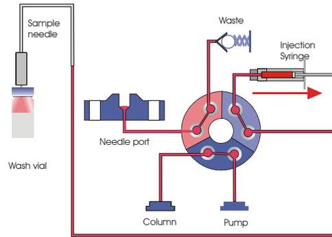
**Fig. 19:** The needle is in the wash vial; the syringe draws a full syringe volume.
