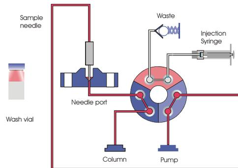
**Fig. 21:** Flow path after PrimeSyringe and with the pump flow turned on again.
