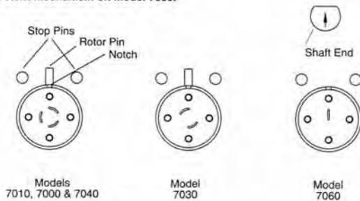
Fig. 6. Correct rotor seal orientation (viewed from stator).
