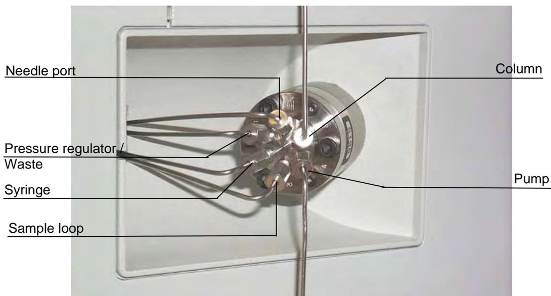
*Fig. 8: Fluid connections*
