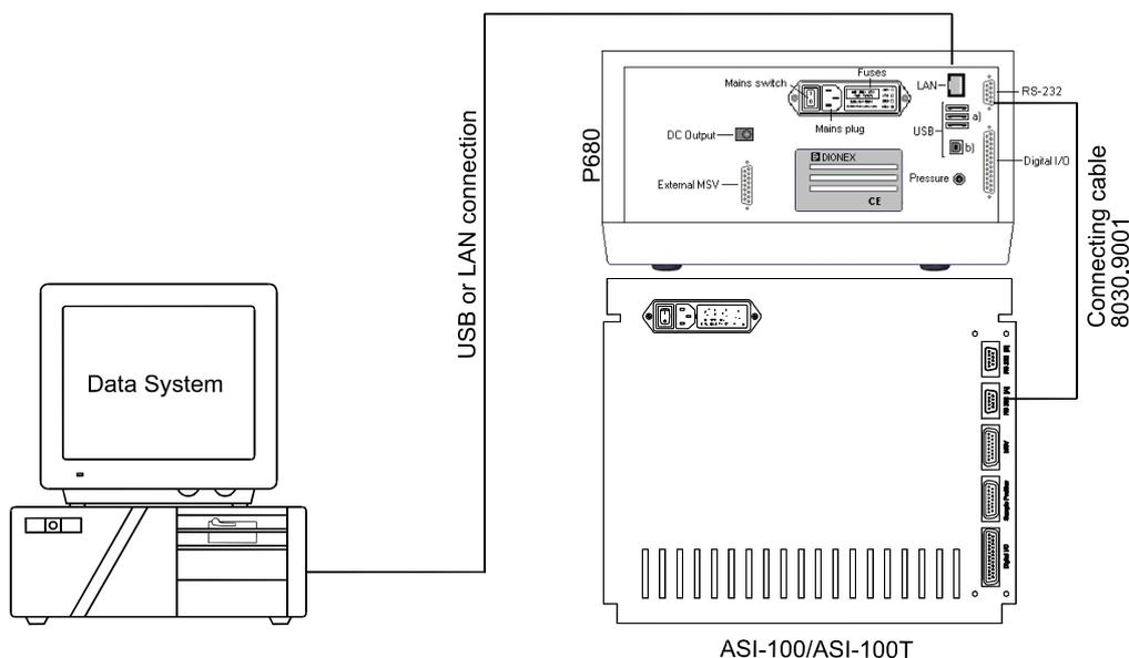
Fig. 11: Autosampler connection to the data system via a P680 pump
