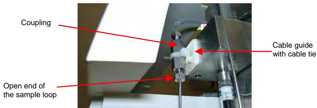
*Fig. 29: Syringe block with cable guide*
