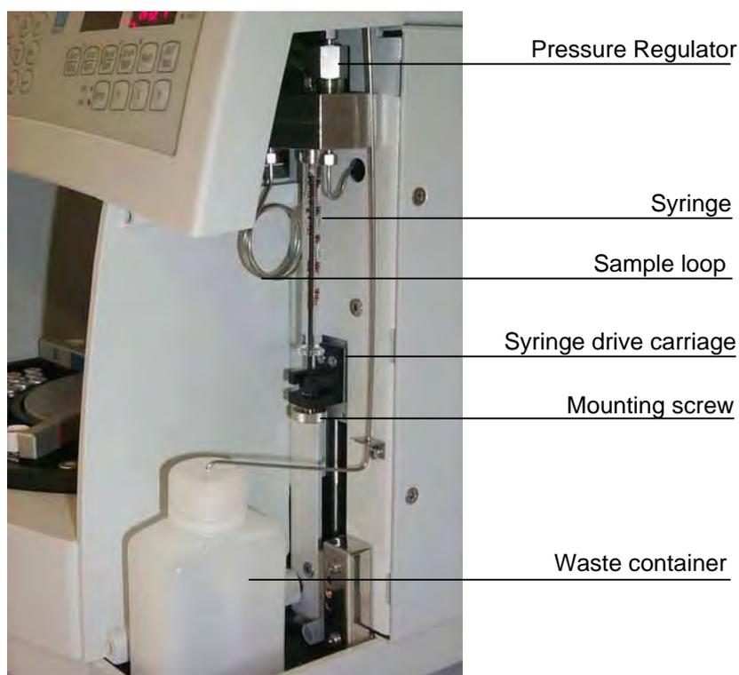
*Fig. 32: Syringe removal/replacement*
