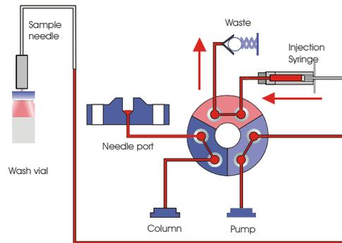
**Fig. 20:** The injection valve is in Inject position; the needle is still in the vial.
