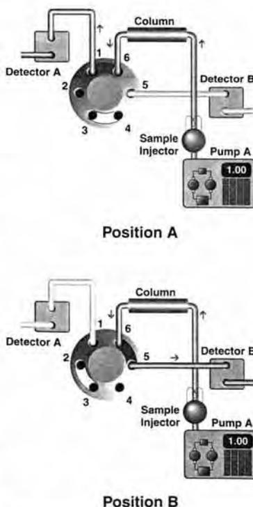
Fig. 9. Diverting flow from one detector to the other using Model 7030.
