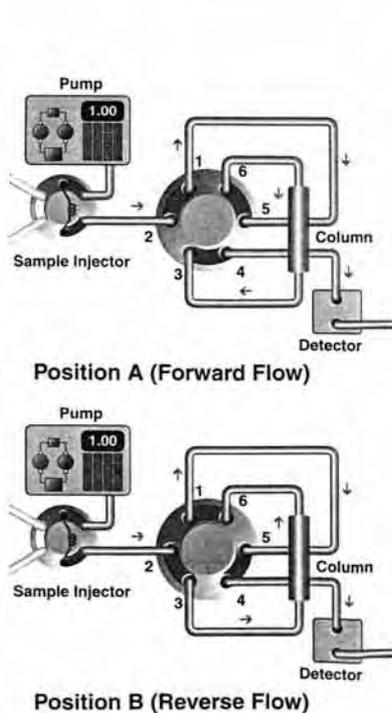
Fig. 8. Illustration of column flow reversal for backflushing using Model 7040.
