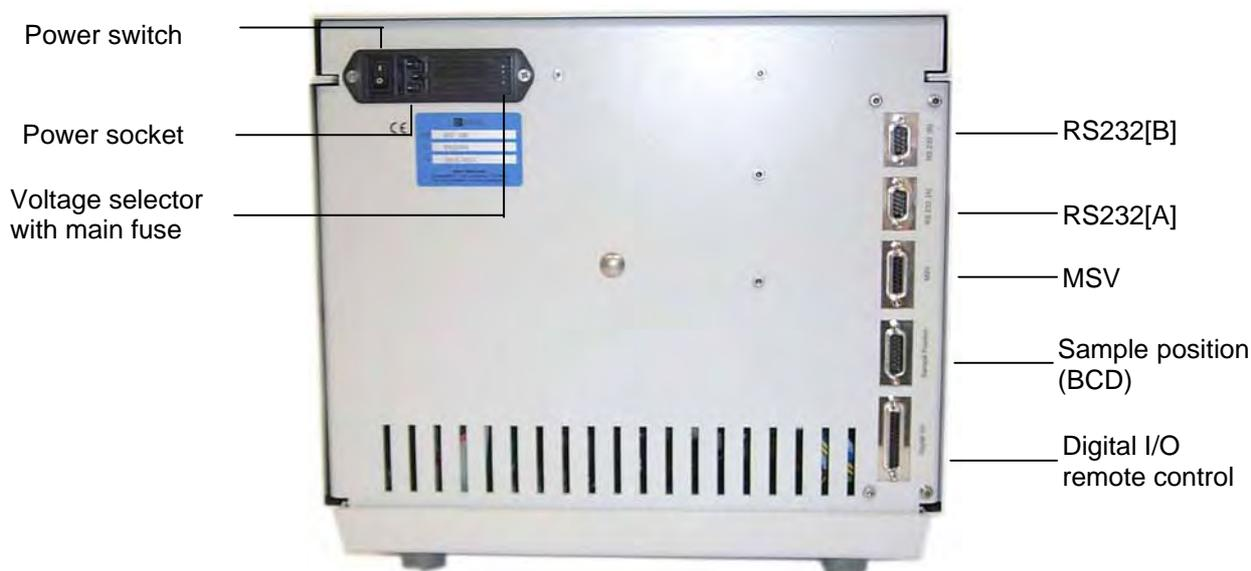
*Fig. 9: Rear panel connections*
