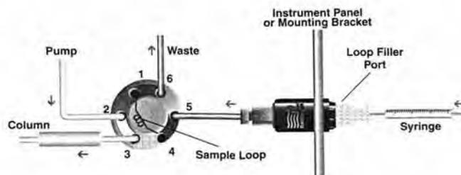
Fig. 3. Using a Loop Filler Port to fill the loop by pressure loading.
