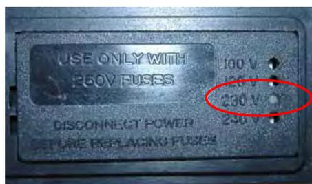
*Fig. 3: Factory-set voltage selection, here: 230V*
