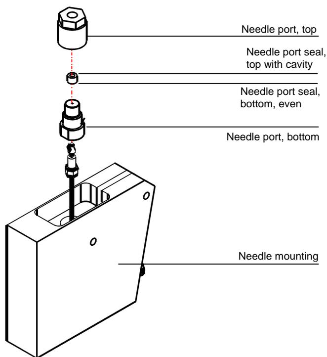
*Fig. 31: Needle port with needle port seal*
