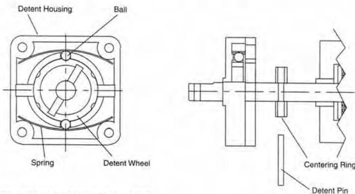
Fig. 5. Detent mechanism on Model 7060.
