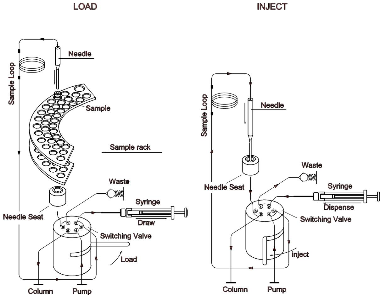
Fig. 1: Injection principle
