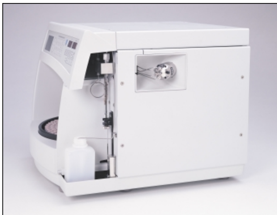
Figure 3. Easy access is provided to the syringe and sample loop.
